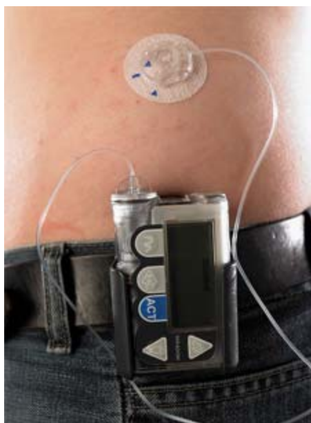
AROUND-THE-CLOCK INSULIN: A portable pump is the most advanced means for delivering insulin. Typically, a pump can be programmed to release a low, steady dose of insulin throughout the day as well as a high dose before a meal. Spikes in blood-glucose levels exacerbate the health complications from diabetes, which can be fatal. Adults with diabetes are two to four times more likely to die of heart disease or stroke than adults without diabetes.
