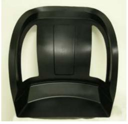
An automotive seat bucket from Fiberforge, a company chaired by Lovins, is ultralight and ultrastrong. Carbon fibers are laid into predetermined positions and sandwiched with reinforcing nylon. The flat, tailored blank is then heated, stamped on a hot molding die, cooled, and trimmed to produce the finished part.
