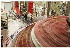
Photo courtesy David Harvey & Carnegie Observatories A rotating furnace at the Steward Observatory Mirror Laboratory at the University of Arizona spin-casts the first mirror for the Giant Magellan Telescope.
