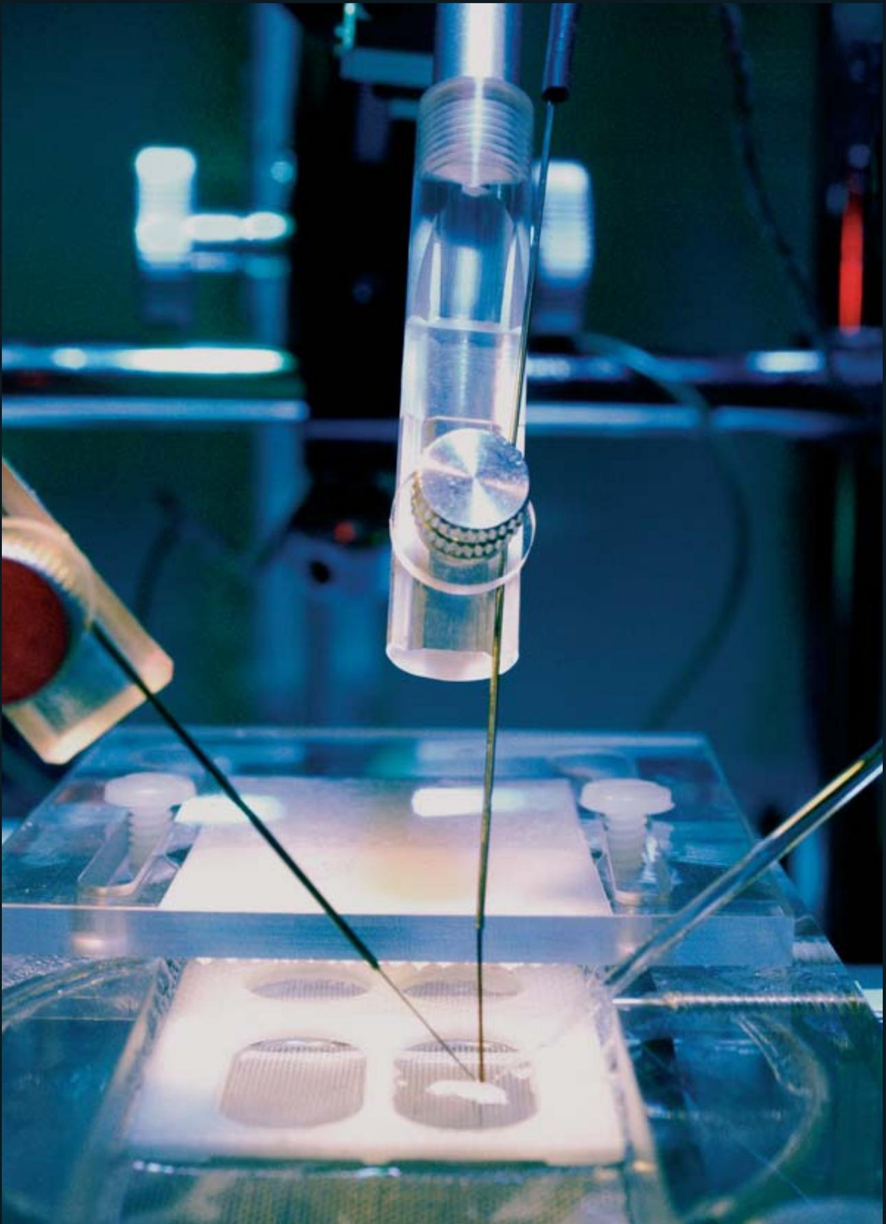
TO SIMULATE MEMORY FORMATION, an electrophysiological recording apparatus can both stimulate and record electrical signals from a 400-micron-thick slice of rat hippocampus.
