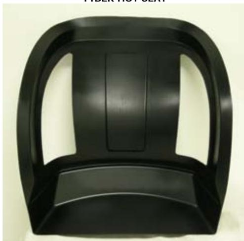
An automotive seat bucket from Fiberforge, a company chaired by Lovins, is ultralight and ultrastrong. Carbon fibers are laid into predetermined positions and sandwiched with reinforcing nylon. The flat, tailored blank is then heated, stamped on a hot molding die, cooled, and trimmed to produce the finished part.
