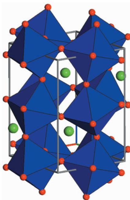
**Figure 1** The structure of silicate perovskite  $(\text{Mg,Fe})\text{SiO}_3$ . Red circles represent oxygen atoms and green circles magnesium or iron. The silicon atoms are located at the centre of the blue  $\text{SiO}_6$  octahedra. Cordier *et al.*<sup>1</sup> add new data on how this material deforms under the conditions of the Earth's lower mantle, and so on anisotropic structures that might be evident with seismological methods.
