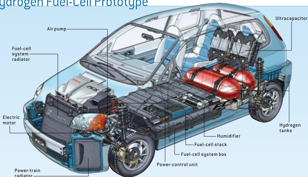
Honda's 2005 FCX model is typical of current hydrogen fuel-cell technology. The four-seat compact, which has a top speed of 93 miles per hour, offers a driving range greater than 200 miles. Equivalent fuel economy is 62 miles per gallon in city driving and 51 mpg on the highway. The FCX's fuel-cell stack, which was designed by Honda for low-cost
