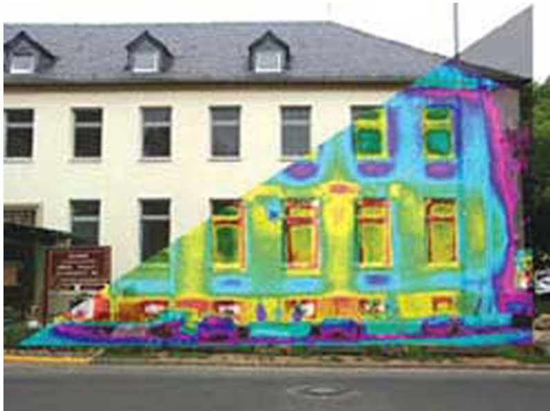
Figure 1.32 A thermograph of part of a building shows temperature variations, indicating where heat transfer to the outside is most severe. Windows are a major region of heat transfer to the outside of homes. (credit: US Army)
